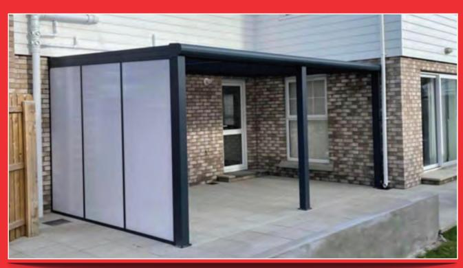
This veranda is fitted in a corner and has one of its ends fitted with polycarbonate panels. In this case it is Opal (opaque) Polycarbonate, but could also be either clear polycarbonate panel or Ultra - Clear panels for greatest transparency.
