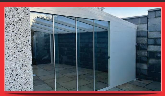
Here the "walk-in" height at the gutter is 1.8m. This 3.7m wide sdewall consists of a 2.5m wide Sliding Glass Panel set (2m high) and a 1.2m wide Solid aluminum panel wall. Note the gutter downpipe exits the corner support post at a height convenient for a water butt.
